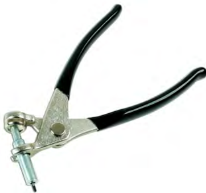
Figure 8-16. Celco pliers ready to insert a 3/32" Cleco fastener.
