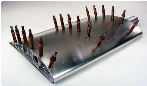
Figure 8-15. A part temporarily held together with Cleco fasteners.
