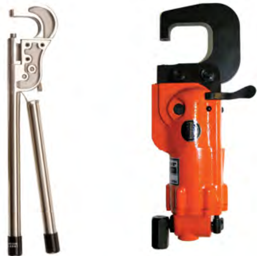
Figure 8-14. Hand and pneumatic type rivet squeezers.
