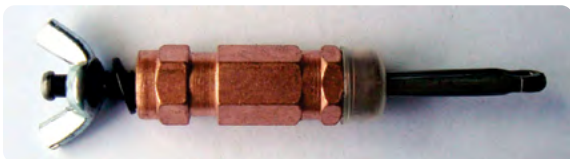
Figure 8-17. A wing nut temporary fastener.
