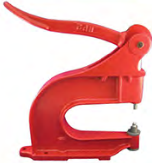
Figure 8-23. Examples of a table riveter and dimpler.
