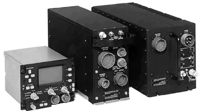
Figure 18-4. Built In Test Equipment (BITE) Indicators.
