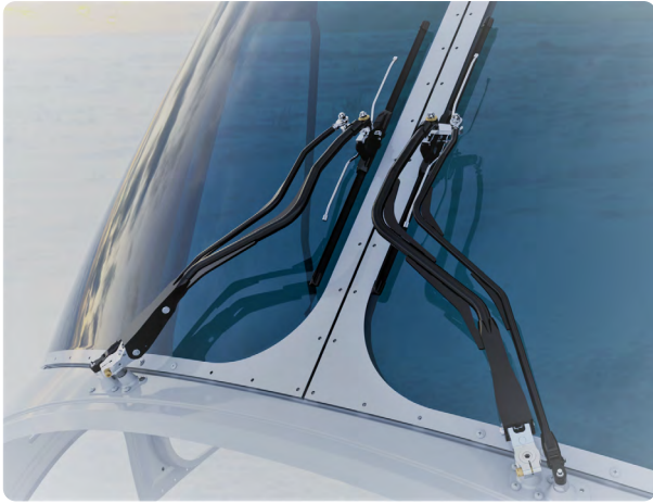
Figure 13-25. An advanced helicopter wash/wipe system by Aerosystems.it depicting dual washer/wiper arms.
