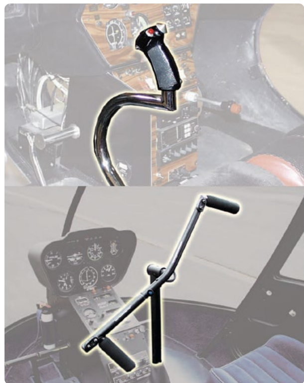
Figure 2-2. Location of cyclic pitch control.
