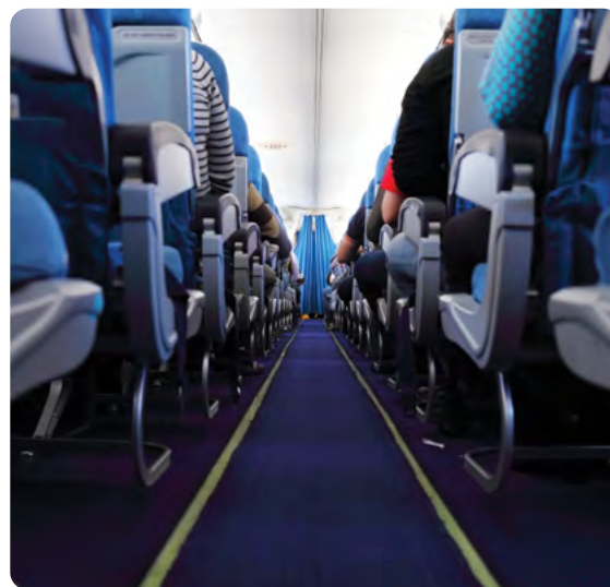
Figure 14-23. Emergency light strips in the aisle floor guide passengers and crew to the exits in case of emergency.
