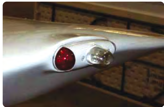
Figure 14-6. A left wing tip position light (red) and a white strobe light.
