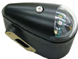
Figure 14-9. A forward position LED position light from Devore Aviation.
