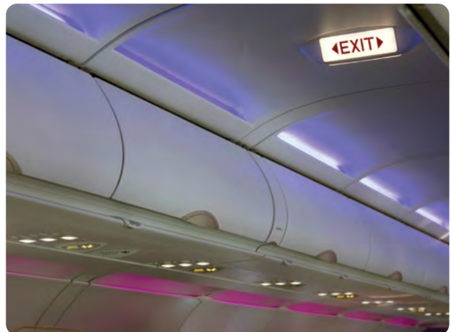
Figure 14-19. Incandescent and fluorescent lights are used to illuminate modern aircraft cabins.
