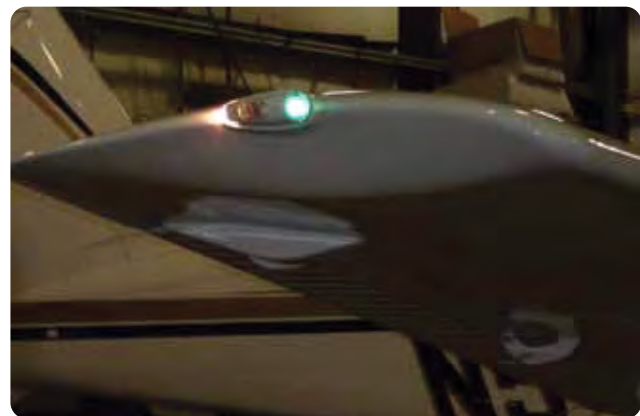
Figure 14-7. A right wing tip position light, also known as a navigation light.
