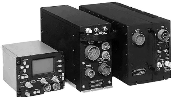
Figure 18-5. Line replaceable units with BITE indicators.
