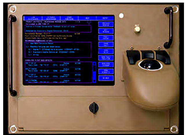
Figure 18-6. Maintenance Access Terminal (MAT).
